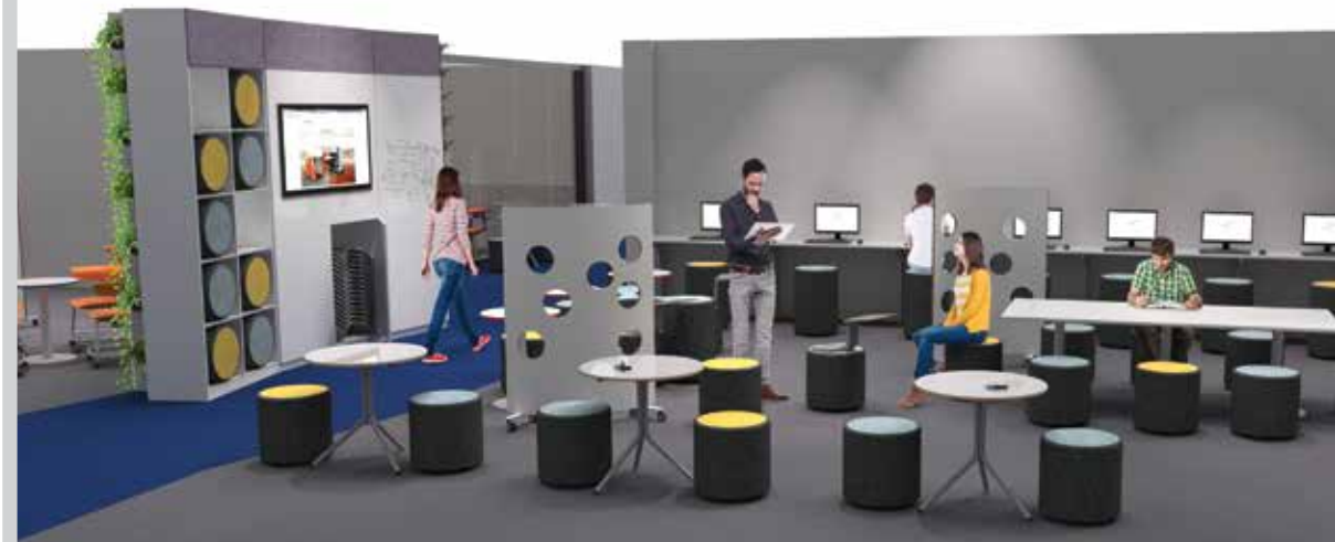
Multi-faceted teacher wall reflects sound back into the learning space / Plant walls improve air quality / Agile furniture creates adaptable spaces / Dry-wipe surfaces increase engagement / Removing walls improves ventilation / Glass walls improve natural light levels and enhance collegiality
